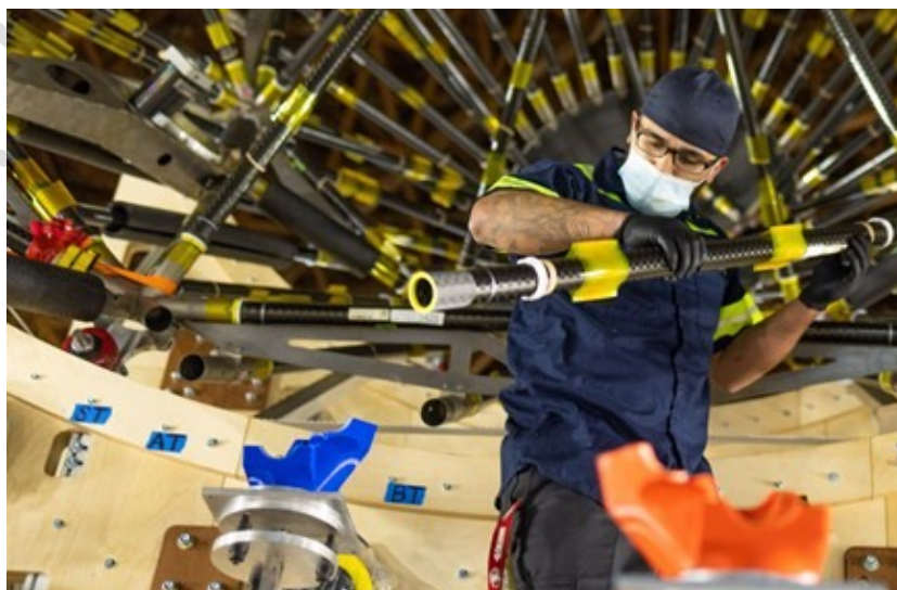
Figure 10: Tube inserted into a Titanium hub (compositesworld)
